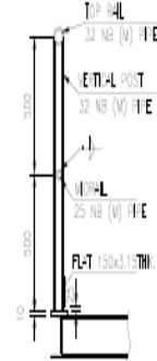
HANDRAIL DETAIL
